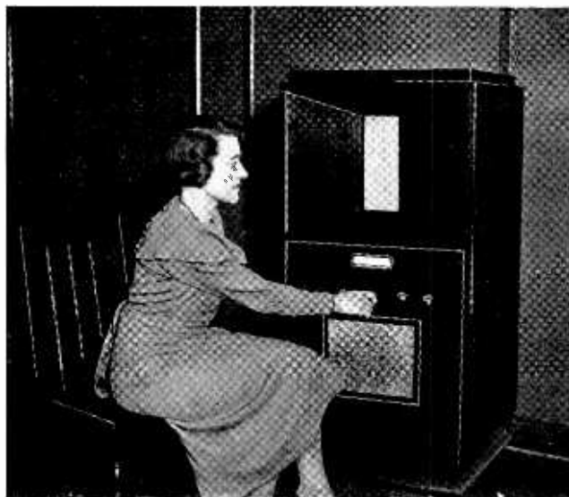
Scophony combined sound and picture receiver for the B.B.C. 30-line transmissions.
