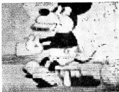
A reproduction of sixty-line horizontal scanning: the stepped effect is apparent.
